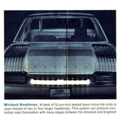
extremes, and can provide excellent coverage of the road and shoulders. The multiplicity of lamps is an added safety factor if any should fail to operate.
