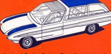
Aerohead Cooling System. The grille air intakes along each side of the hood permit air in the engine compartment to be sucked out by the air stream over the hood, thereby increasing the air flow through the radiator. This permits the use of a small radiator core to provide efficient cooling, thus allowing a more aerodynamic frontal design. Heat Reflecting Roof. The portion of the roof behind the roll bar is of textured, aluminum material that reflects infra-red rays.
