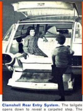
liftgate swings up with the aid of torsion bars and slides back over the roof by means of a sliding track mechanism to permit easier entry. Children's Compartment. This thoroughly equipped area can be sound-isolated from the rest of the interior by power-operated glass.
