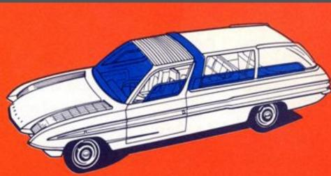
Wrapover Windshield. The windshield "wraps" well into the roof, where it meets the polarizing sun roof. This affords excellent overhead visibility, even when the adjustable roof is in its opaque position. Jalousie Windows. Nearly flush jalousie windows provide smoother air flow and reduced wind noise. Safety Rollover Bar. The roll bar, which separates the polarizing sun roof from the heatreflecting rear roof, is an integral part of the body design.
