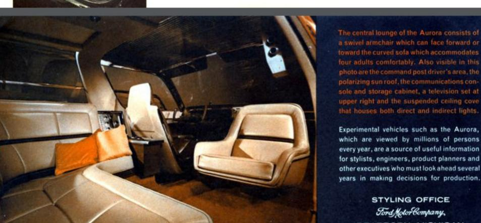
a swivel armchair which can face forward or toward the curved sofa which accommodates four adults comfortably. Also visible in this photo are the command post driver's area, the polarizing sun roof, the communications console and storage cabinet, a television set at upper right and the suspended ceiling cove that houses both direct and indirect lights. Experimental vehicles such as the Aurora,
